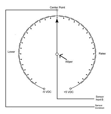
Figure 3-7: Typical OEM Potentiometer with -5 to +5 VDC Power
